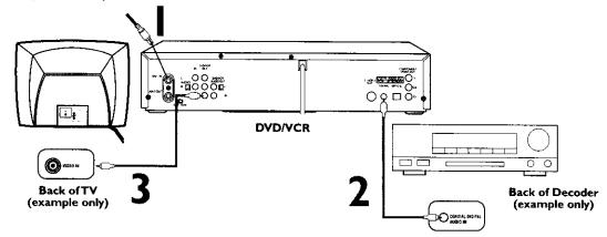
Connect the antenna or cable to the ANT-IN (Antenna In) jack of your DVD/VCR.
